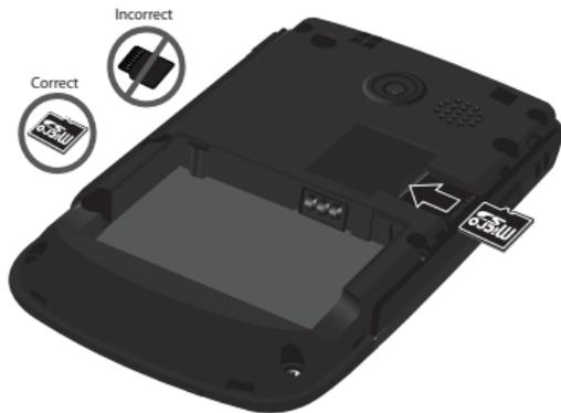
3. Press the memory card into the slot until the card locks into place.
